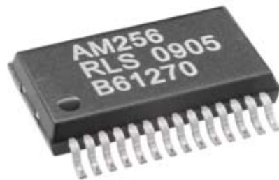
AM256 magnetic encoder chip combines ruggedness and performance
