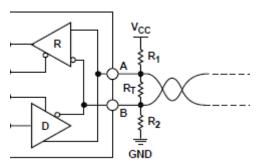
**4. Cable Selection:** When wiring RS-485 lines, it is important to use twisted pairs on the 485+/485- lines to increase noise immunity. See below.
