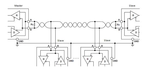
Note: If the communication bus is very short, then the termination resistor may drown out the signal entirely. In this case, a termination resistor should not be used.
